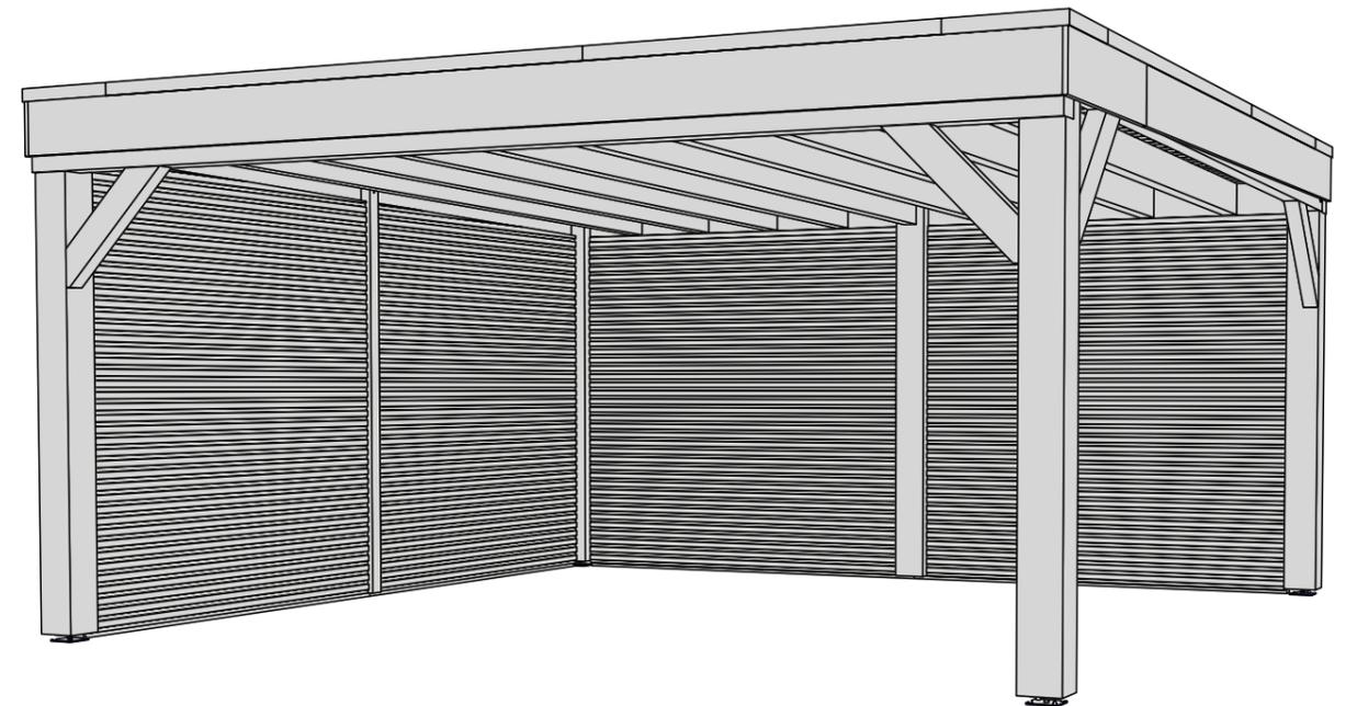
PREVOIR PLOT DE SUPPORT INTERMEDIAIRE SI L'ABRIS N'EST PAS POSE SUR DALLE
